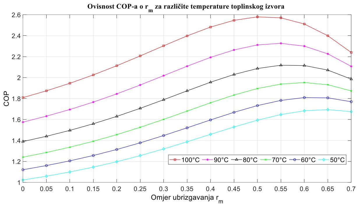
**Slika 48. Ovisnost COP-a o  $r_m$  – Temperatura toplinskog ponora 158,83 °C**
