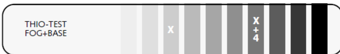
Slika 11: Certificirani pred-eksponirani film (certified PMC-strip)
