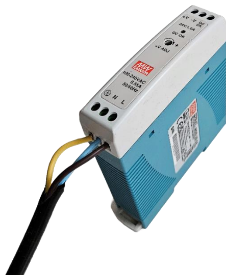
Slika 4.2 Napajanje Mean Well MDR–20–24
