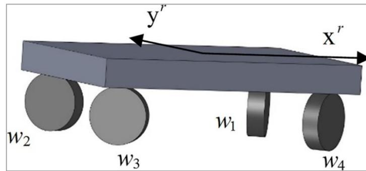
**Slika 2. 4WIS4WID sustav robota [2]**
