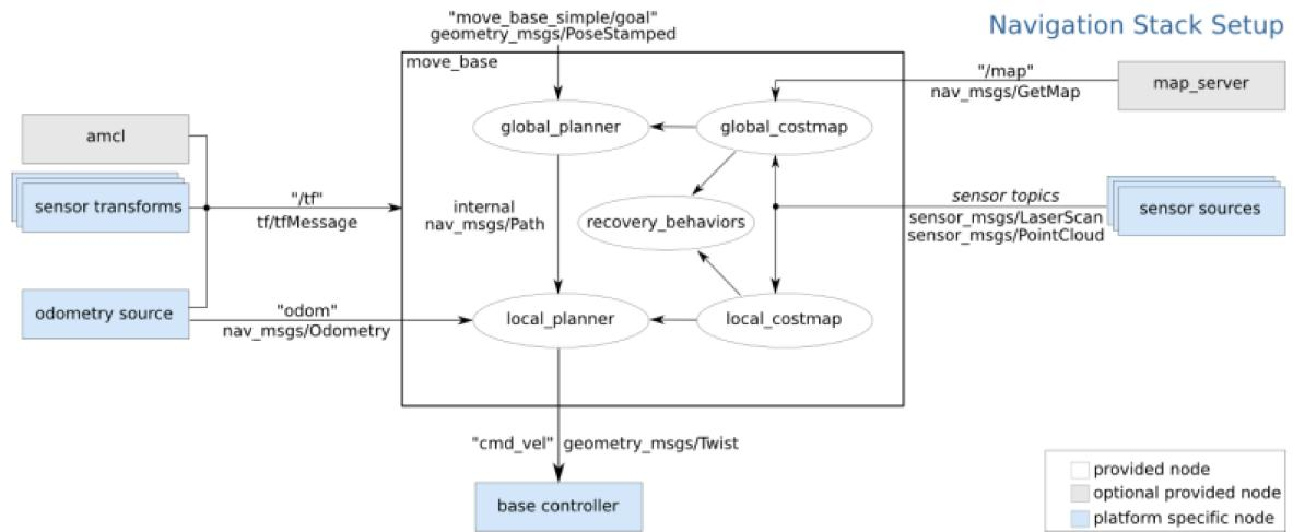
Slika 7.1: Blok dijagram rada *navigation stack-a* [30]
