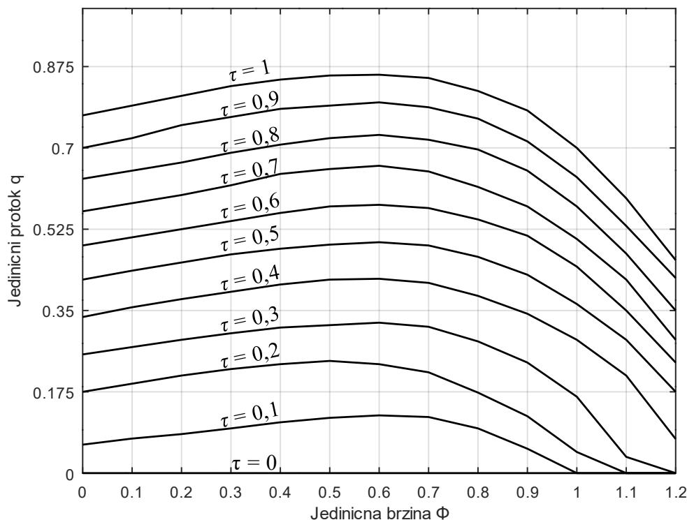
**Slika 13. Karakteristika protoka**
