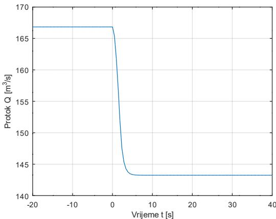
**Slika 21. Protok nakon zatvaranja**
