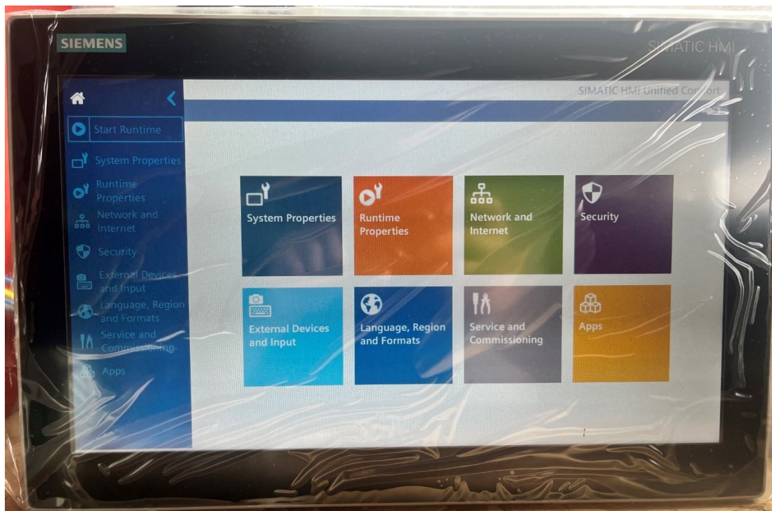
Slika 4. SIEMENS HMI MTP1500 Unified Comfort panel
