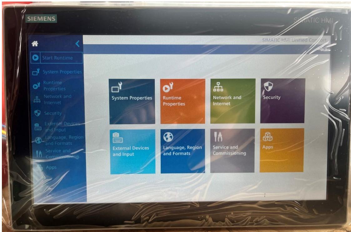
Slika 4. SIEMENS HMI MTP1500 Unified Comfort panel
