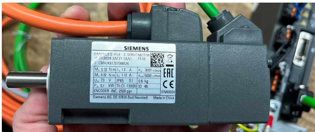
Slika 7. SIMOTICS S-1FL6024-2AF21-1AA1 servo motor
