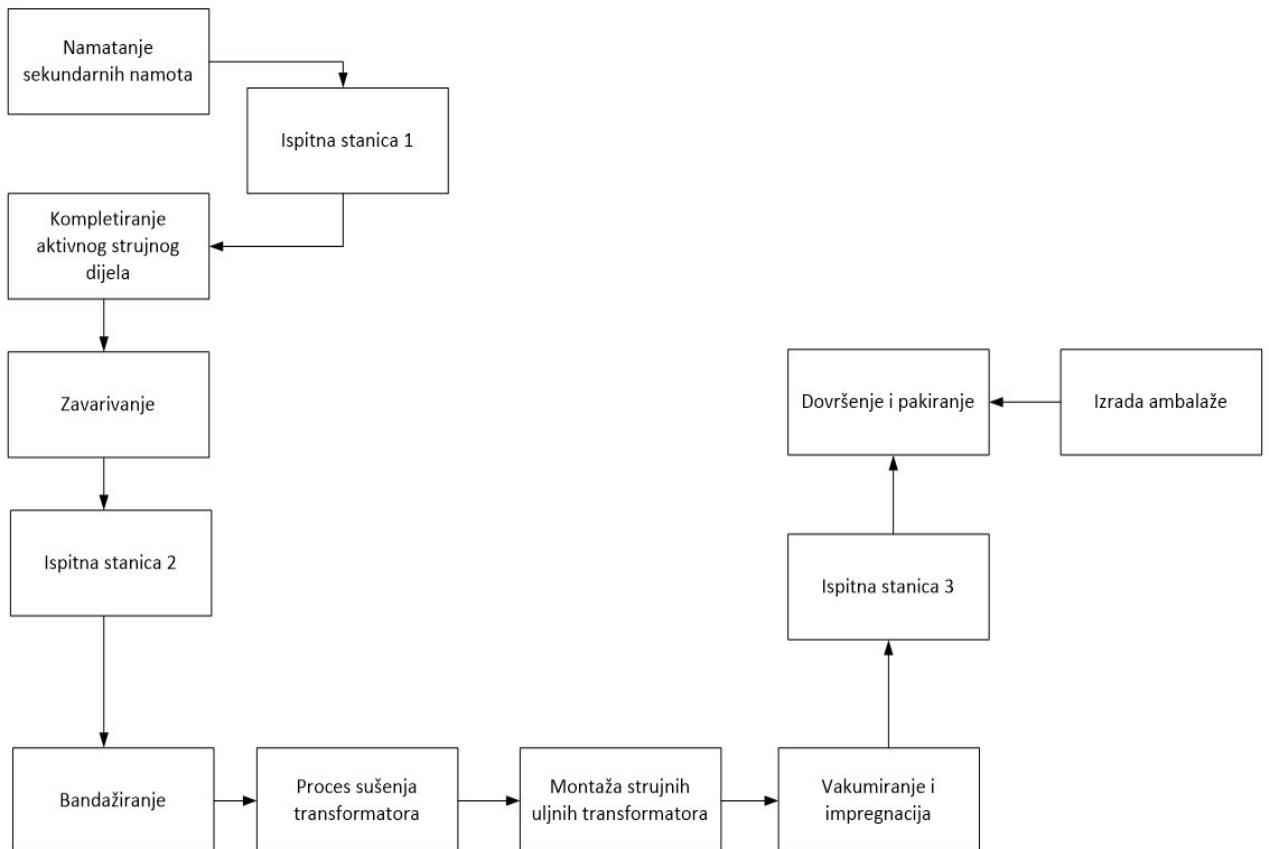
Slika 3.2 SHEMA IZRADE ULJNIH STRUJNIH TRANSFORMATORA TIPO AGU
