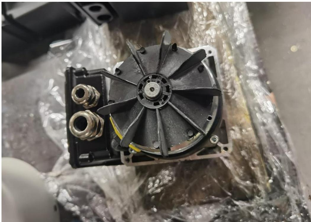
Slika 9. Ventilator servomotora
