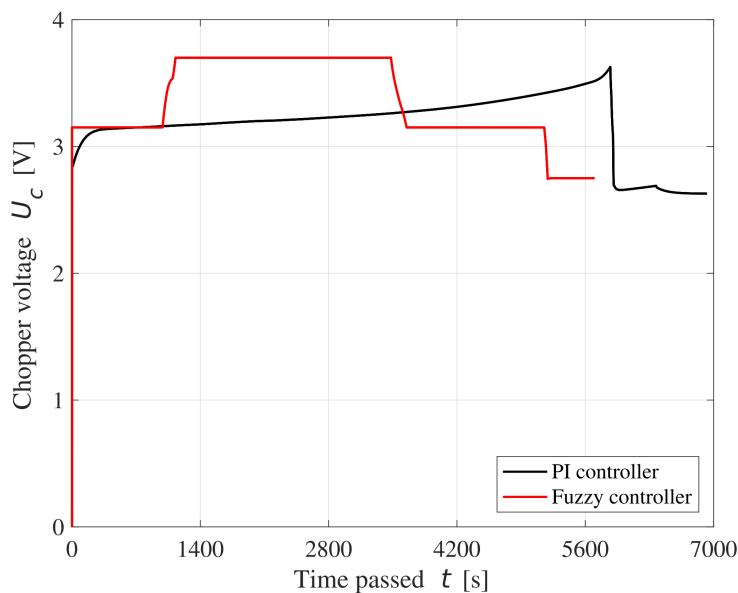
Slika 47: Napon pretvarača; PI vs Neizraziti regulator
