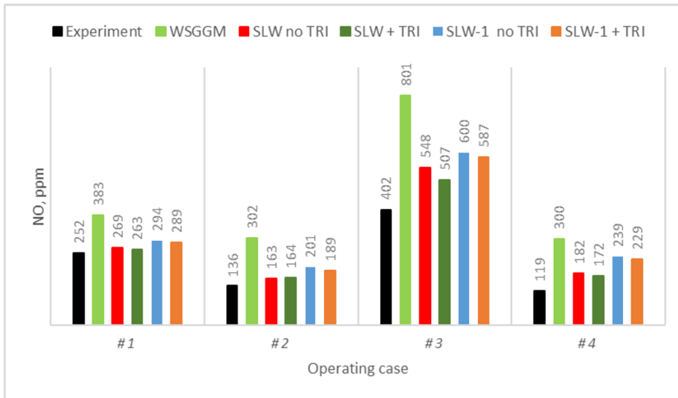
Figure 42 NO results at the exhaust system for ICE cases
