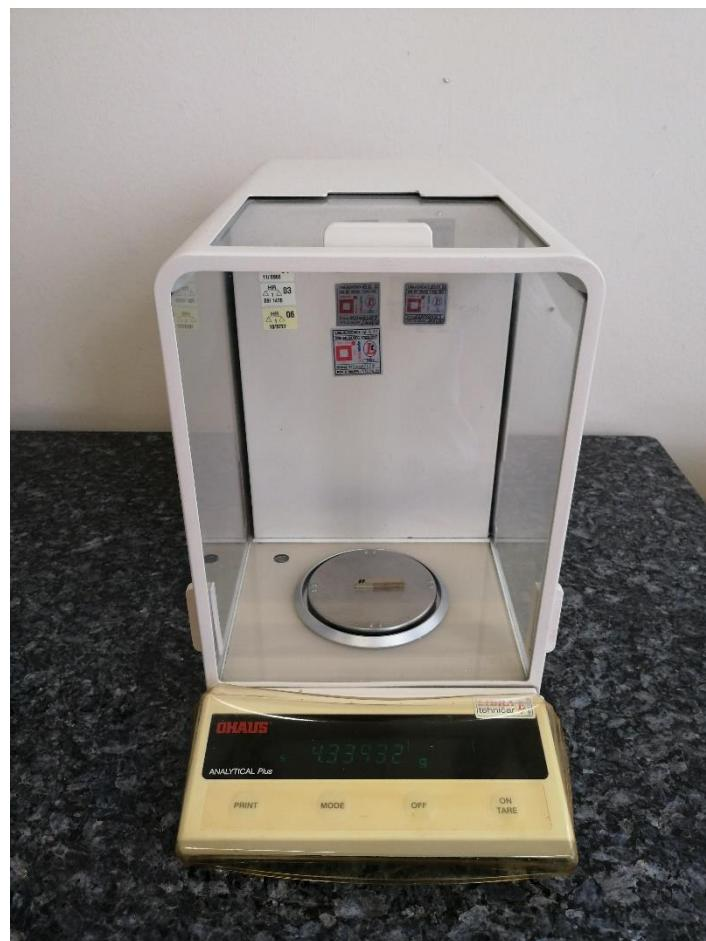
Slika 36. Mjerna vaga "Analytical Plus balance Ohaus"
