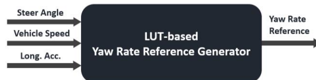
Figure 26. Proposed LUT-based yaw rate reference generator
