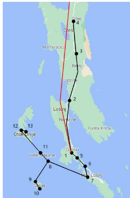
Figure 23 The topology of the observed distribution system – red line represents a transmission 110 kV line to Krk island, black lines are the distribution lines and black nodes are the distribution transformers 10(20)/0.4 kV
