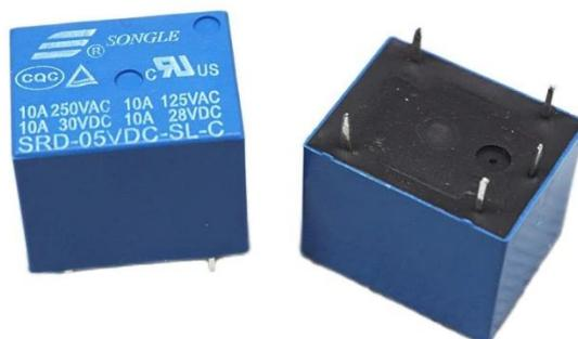
Slika 11. Relej SRD-05VDC-SL-C
