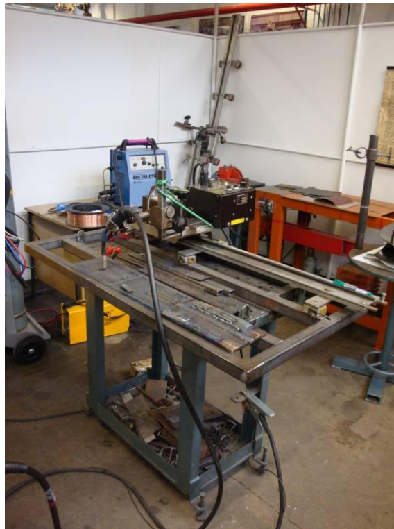
Slika 7. Automat BUG – O Systems, MOD. BUG – 5300.
