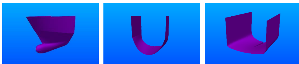
Figure 10. Hull modules used within the proposed design procedure (fore, mid and stern modules).
