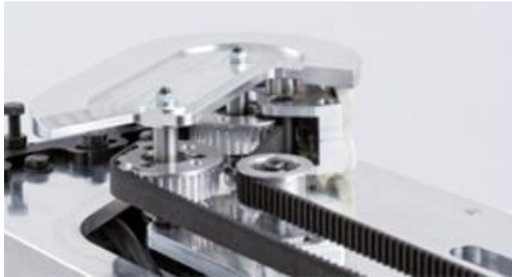
Slika 12. Bode - SST electric sliding plug doors, zupčasti remen [14]
