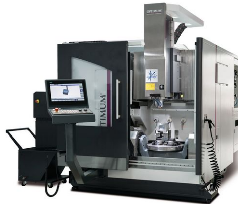
Slika 1.2: Petoosna glodalica OPTImill FU 5-600 HSC 24 [3]
