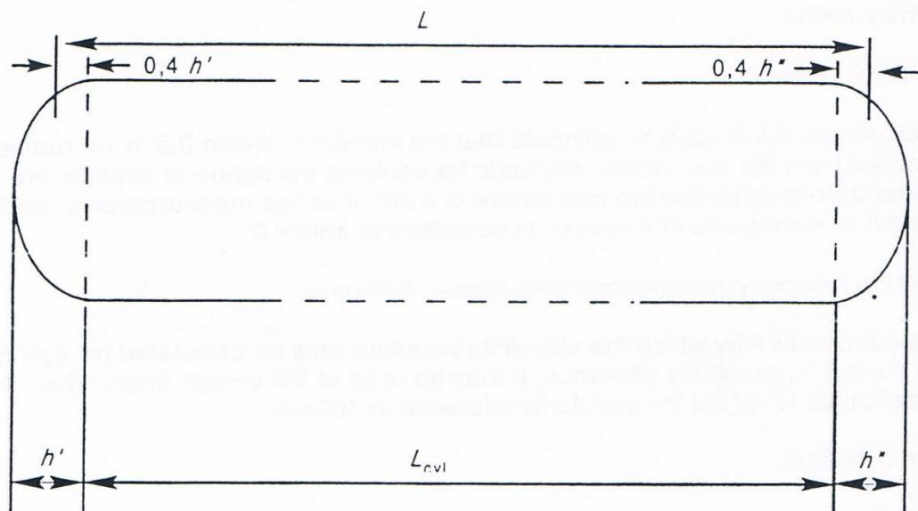
**Figure 8.5-1 : Cylinder with heads**
