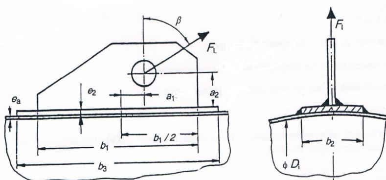
Figure 16.7-1 : Longitudinal lifting eye
