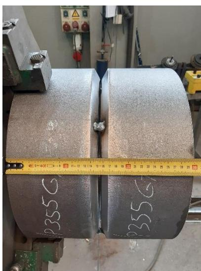
**Slika 41. Epruveta V-1 prije zavarivanja**
