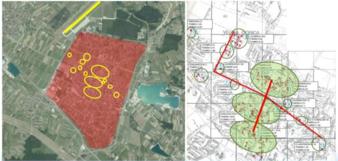
Figure 1 Group of smaller district heating systems
