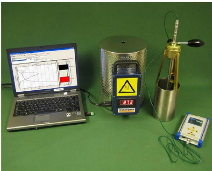
Slika 5.9 Mjerni sustav IVF Smart Quench System (ISO 9950) [30]
