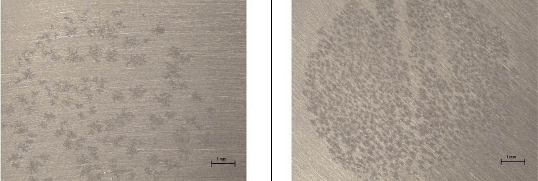
Two side-by-side micrographs showing the surface of sample C11. The left image shows the surface after Tafel extrapolation, and the right image shows it after cyclic polarization. Both images show a textured surface with small, dark, irregular spots. A 1 mm scale bar is present in the bottom right of each image.   |                             |
