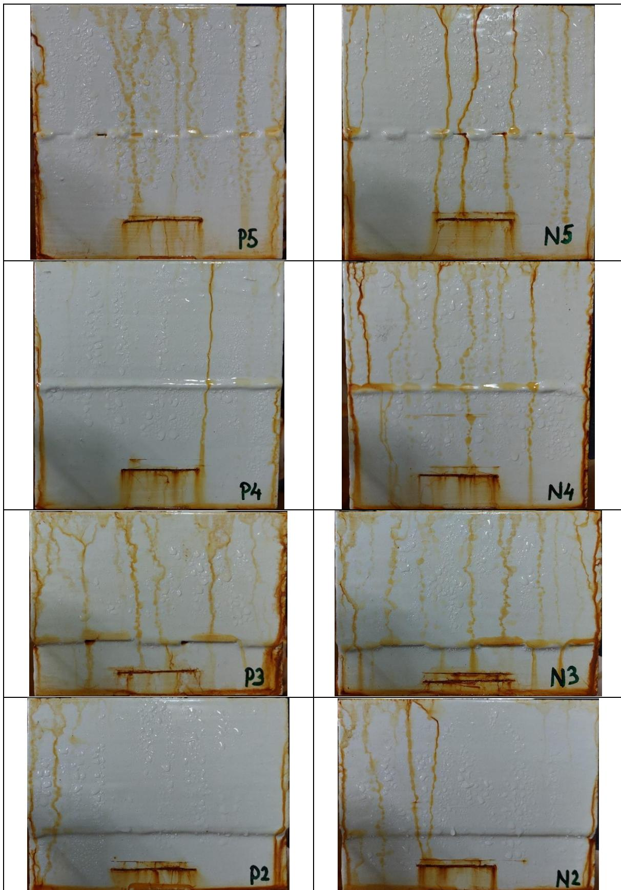
**Tablica 9. Ispitivanje u slanoj komori nakon 384h**
