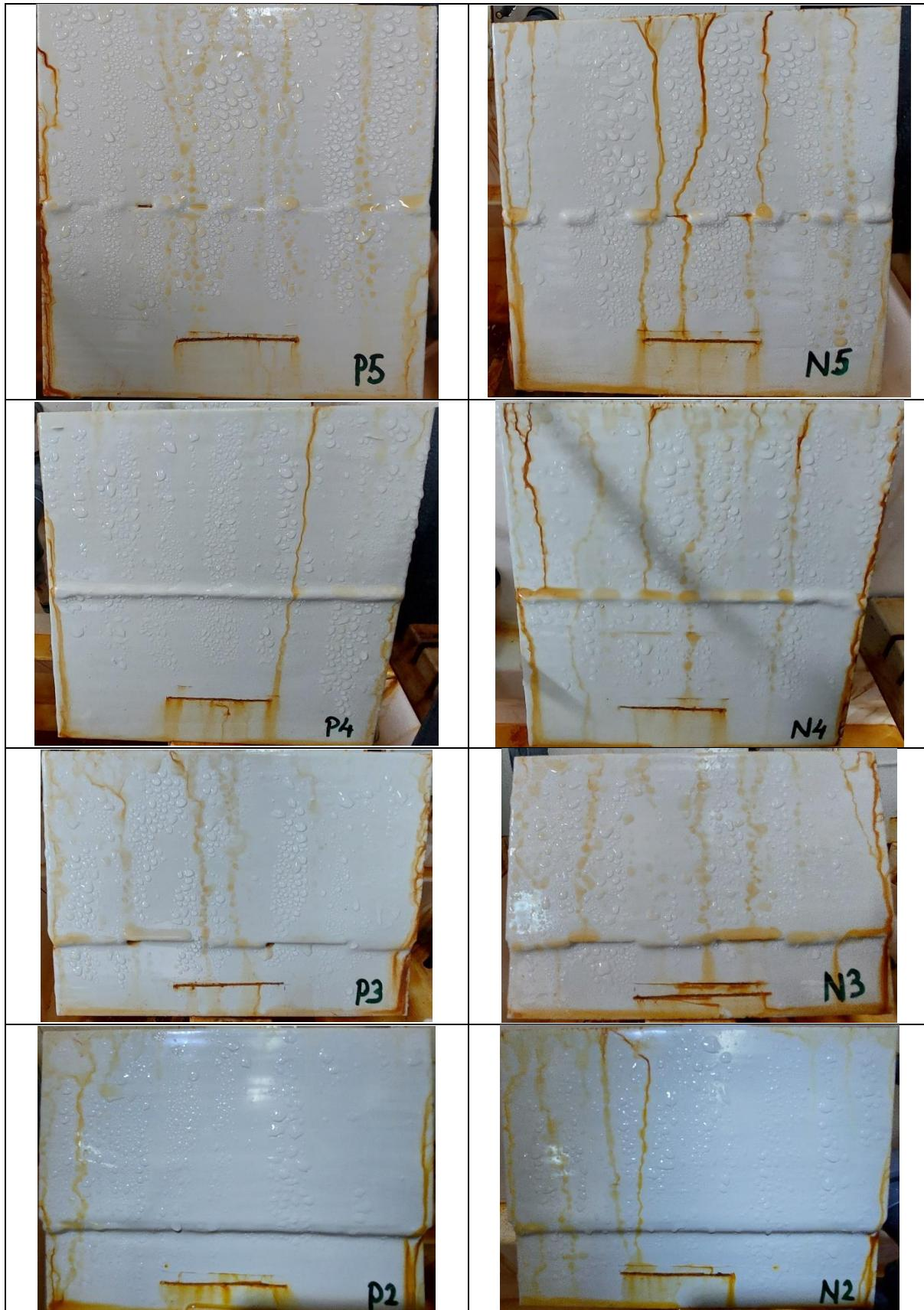
**Tablica 8. Ispitivanje u slanoj komori nakon 192h**
