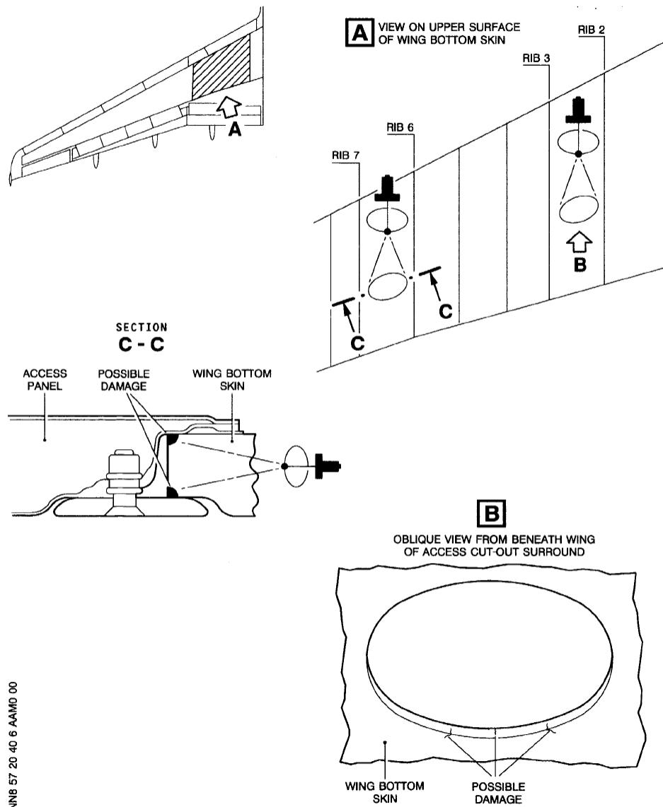
Inspection Area with Possible Damage
