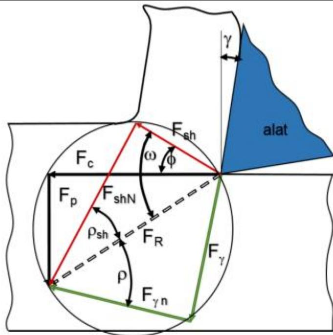
Slika 10. Merchantov model sila rezanja [9]
