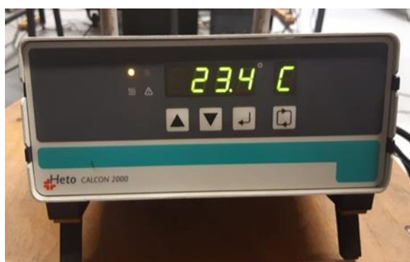
Slika 2. Regulator temperature, Heto Calibration CALCON 2000
