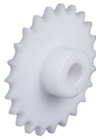
Sprocket KRK with hub 08 B-1 1/2 X 5/16" 25 teeth material polyacetal resin
