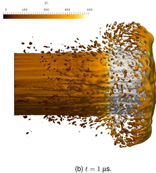
Figure 13: Side view of the atomization onset at the two time steps.
