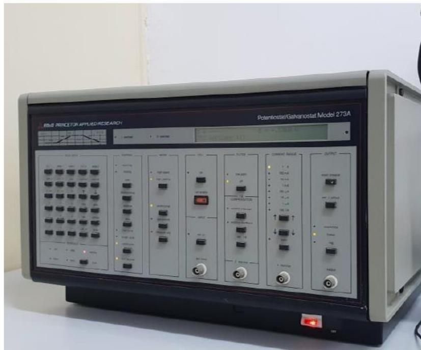
Slika 39. Potentiostat/Galvanostat Model 273A EG&E
