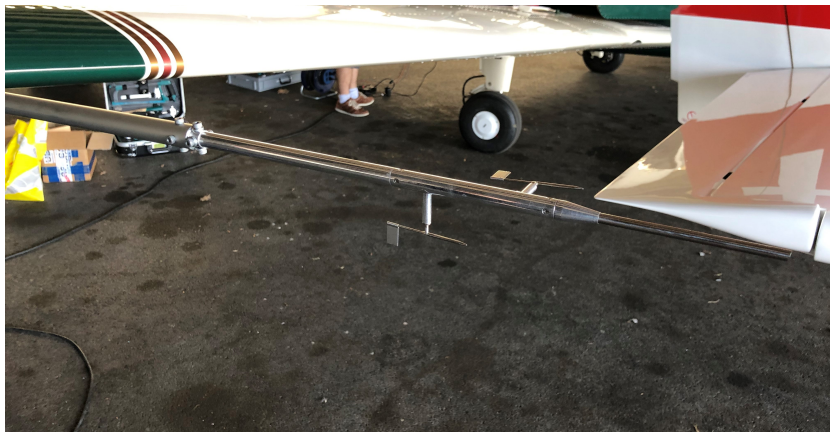
Figure 2.3: Air Data Boom (ADB) [1]
