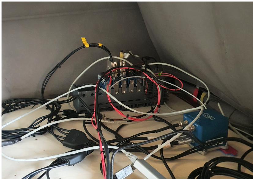
Figure 2.5: Real-time embedded industrial controller (cRIO)
