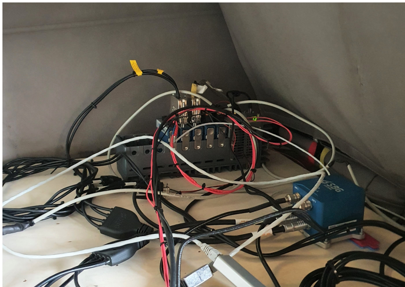
Figure 2.5: Real-time embedded industrial controller (cRIO)
