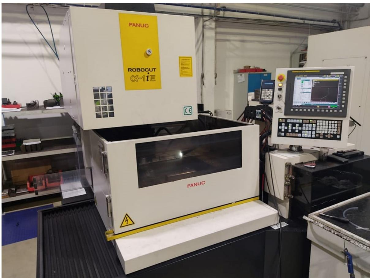
Slika 54. EDM Wire Fanuc Alpha 1i E
