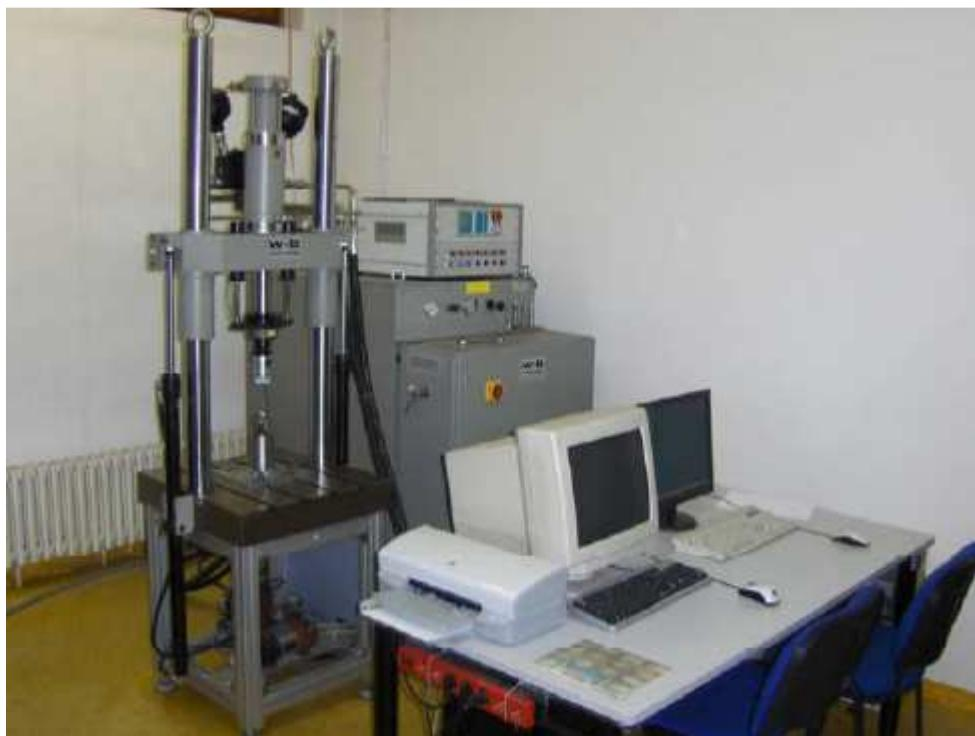
Slika 4.6 Servohidraulička kidalica LFV 50-HH, Walter+Bai
