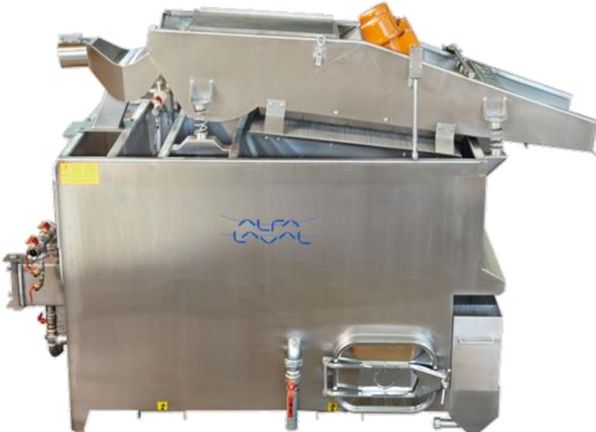
Slika 2.7. Alfa Laval Olive compact washer with defoliator [15]
