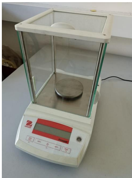
Slika 30 Vaga Pioneer Ohaus Analytical Balances
