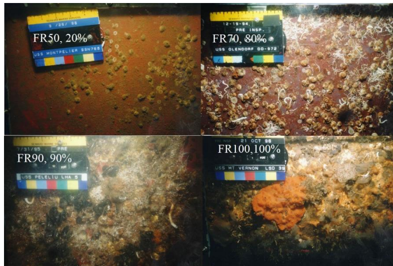
Figure 1.3 Fouling rating scale for hard and composite fouling [40]
