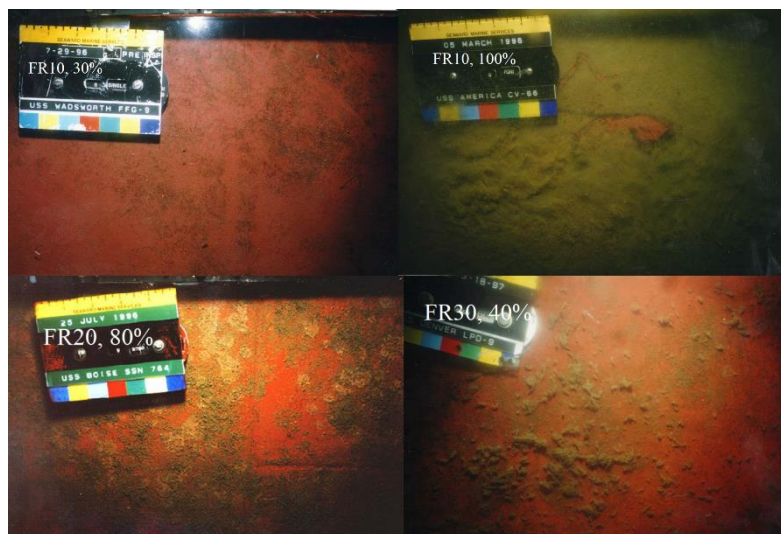
Figure 1.2 Fouling rating scale for soft fouling [40]
