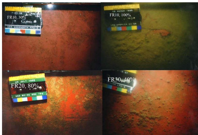
Figure 1.2 Fouling rating scale for soft fouling [40]
