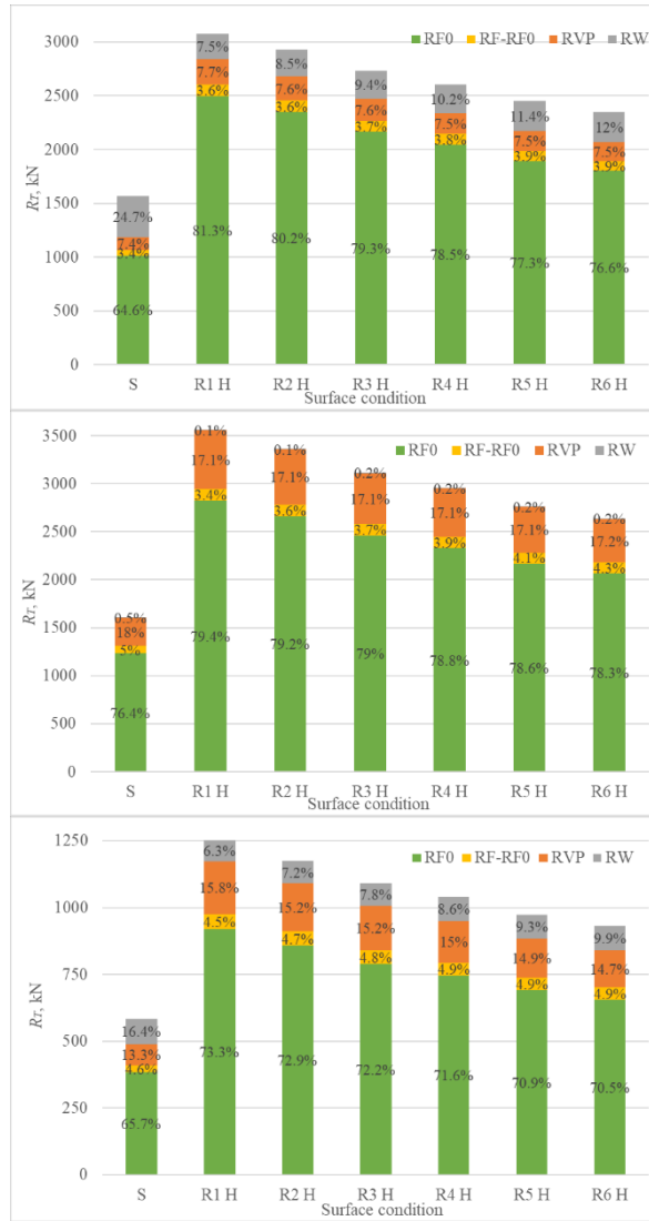
Figure 5.22 The decomposition of R_r for KCS (upper), KVLCC2 (middle) and BC (lower) fouled with hard fouling
