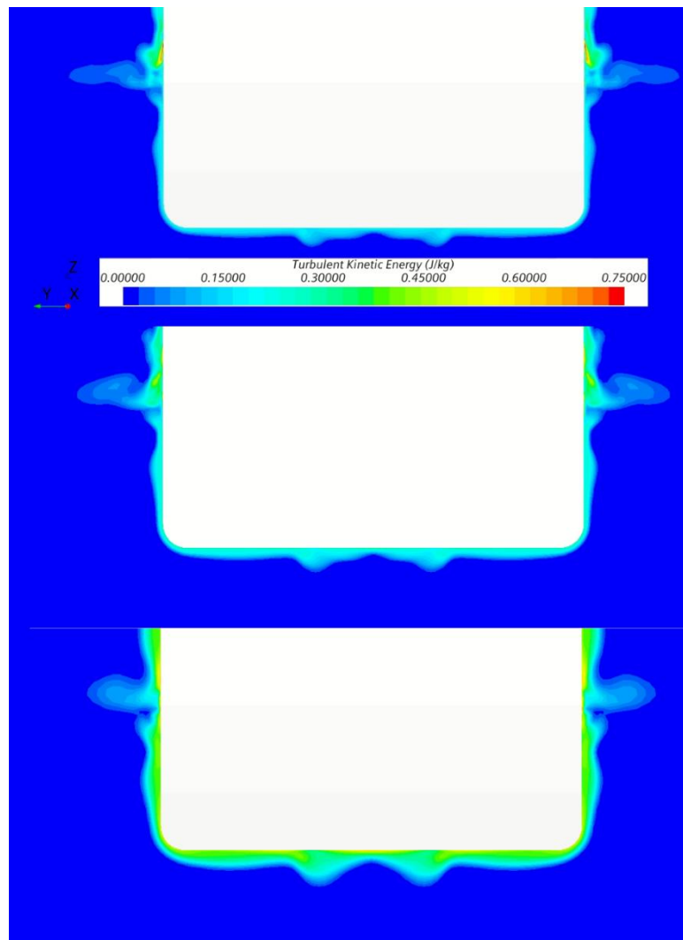
Figure 5.31 The obtained turbulent kinetic energy contours for smooth KCS hull (upper), KCS with R2 B (middle) and KCS with R1 H (lower) at the midship plane
