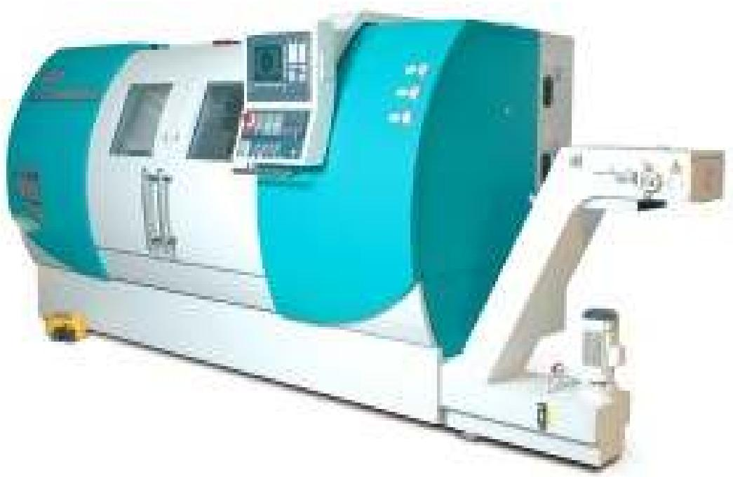
Slika 4.2 tokarski obradni centar Trems SBL-500 [16]
