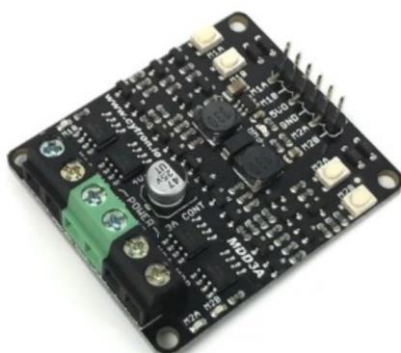
Slika 4.4. Cytron 3A 4-16V Dual Channel DC Motor Driver[12]
