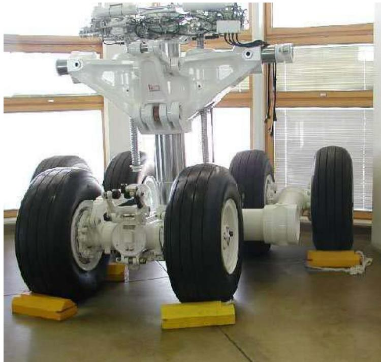
Slika 17: Stajni trap Lockheed C-5A
