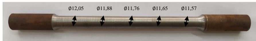
**Slika 5.2. Promjeri uzorka**
