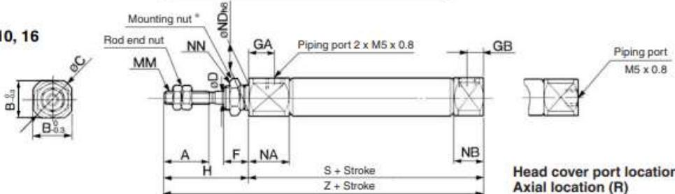
With air cushion: CJ2B [Bore size] [Stroke] A [Head cover port location]
