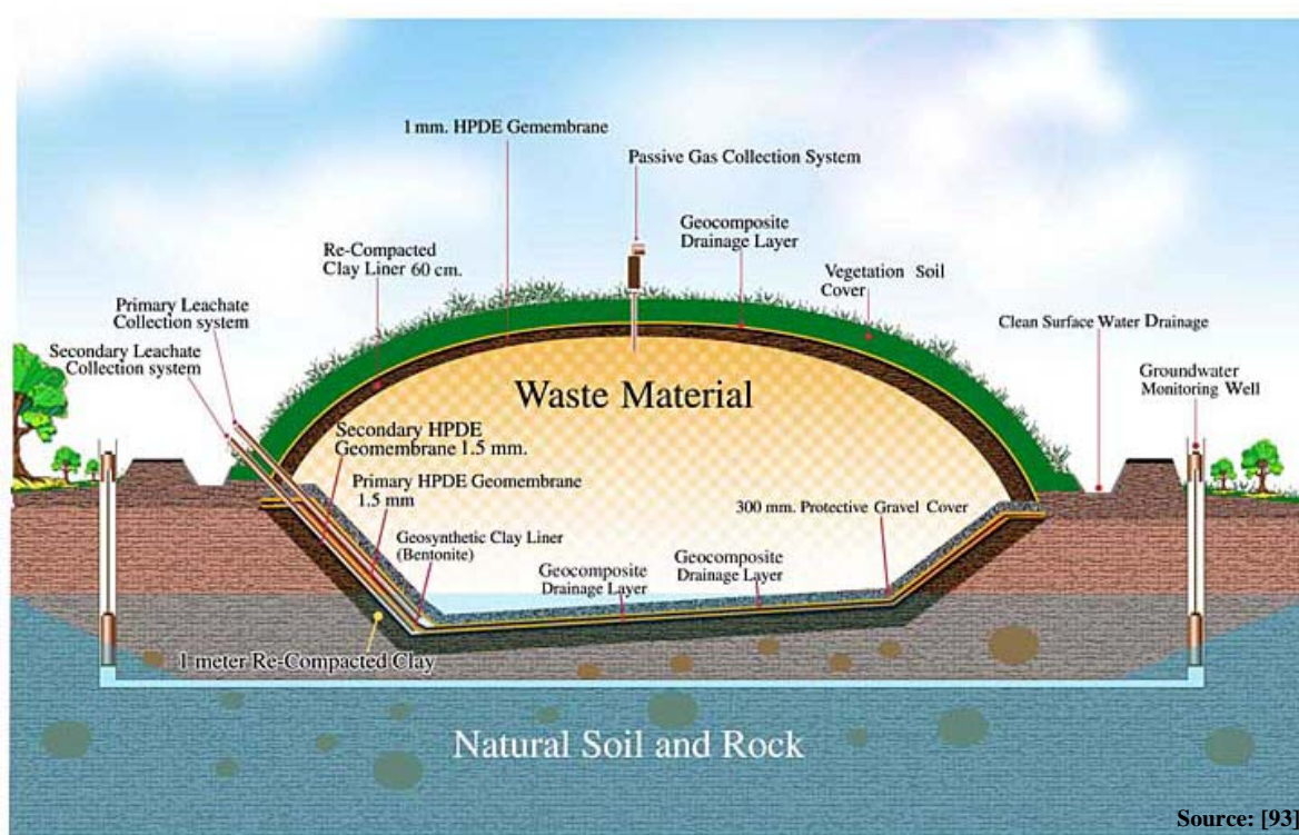
Figure 2-14: Engineered Landfill
