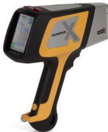
Slika 28: Rendgenski fluorescentni spektrometar Olympus DELTA Professional [39]
