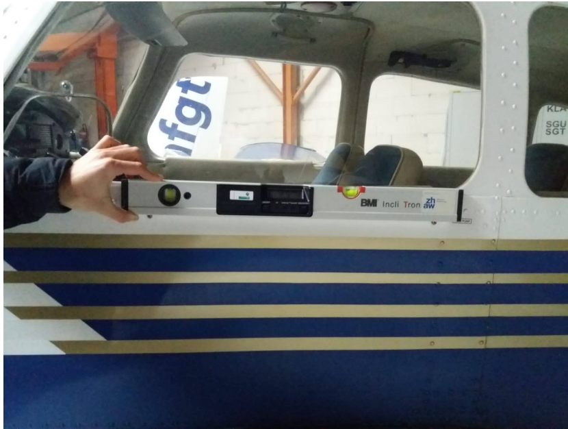
Figure 6.1: Measuring the water line level of the aircraft
