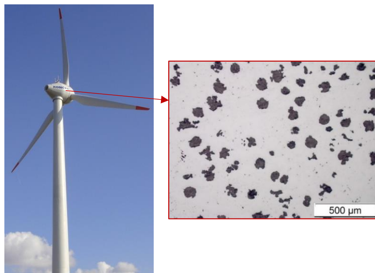
Fig. 1.1. Example of microheterogeneous materials used in modern-day engineering (Končar KO VA 57/1 wind turbine with nodular cast iron hub)
