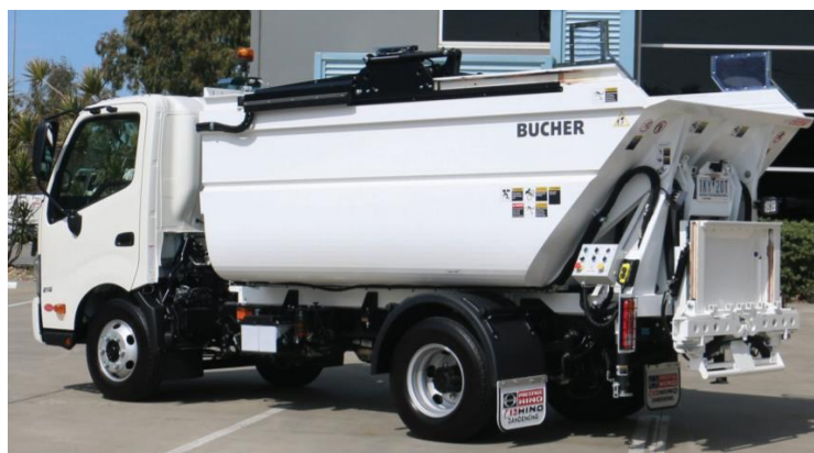
Slika 29. Bucher Municipal Satellite Rear Loader [35]
