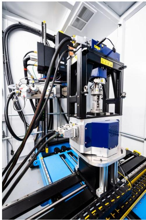
**Slika 3.5 Deben CT20kN Open Frame Test Rig [13]**
